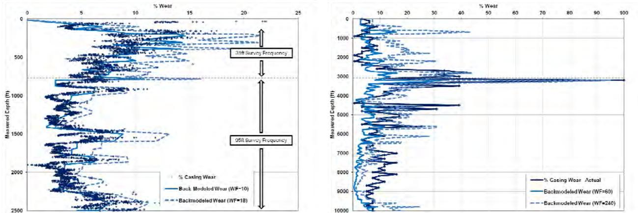
**Figures 7 and 8. Casing wear back-model results for a S-shape land well in the western US, and a horizontal well in North Dakota. Notice that in both of these wells, the maximum wear is far greater than predicted when the average wear is matched up.**
