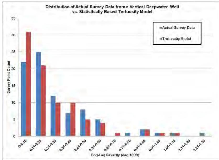
**Figure 11. Comparison of the distribution of dog-leg severity of an actual vertical deepwater well and the results from a tortuosity simulation using the gamma distribution model described in this paper.**
