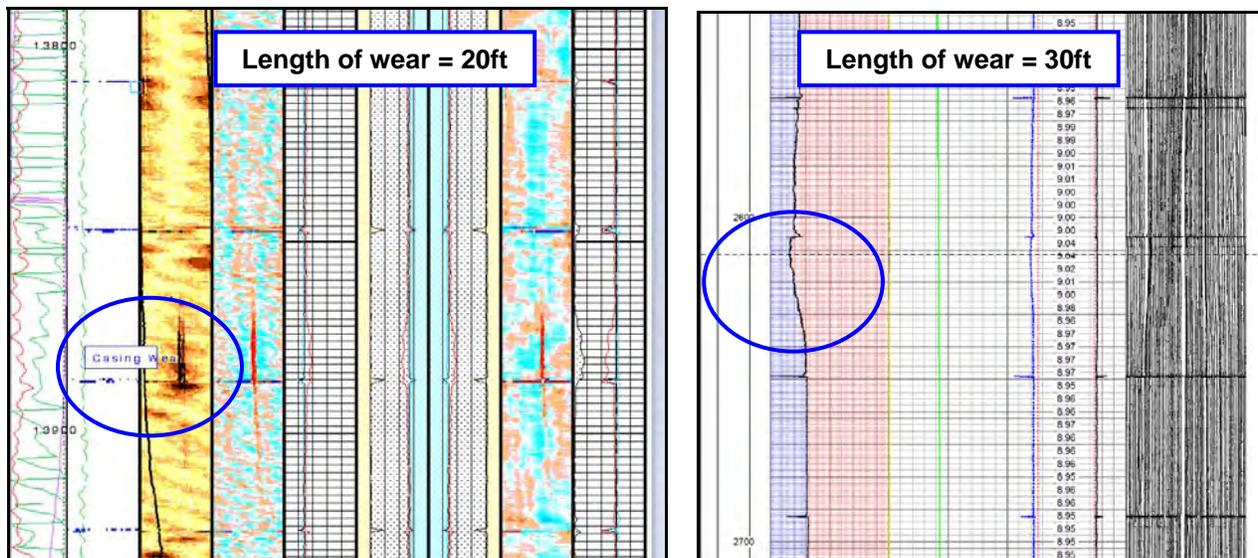
Figures 9 and 10. Examples of casing wear logs showing acute, short distance wear.
