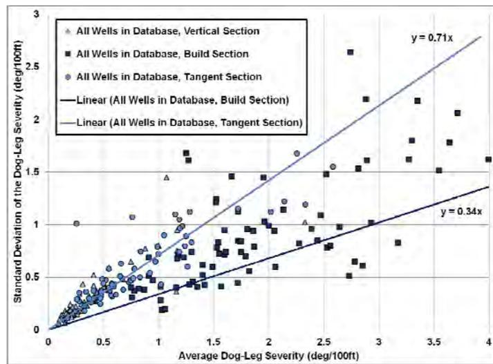
Figure 3. Graph showing the average vs. standard deviation of dog-leg severity for wells used in this database to illustrate that the standard deviation increases with increasing build rate.
