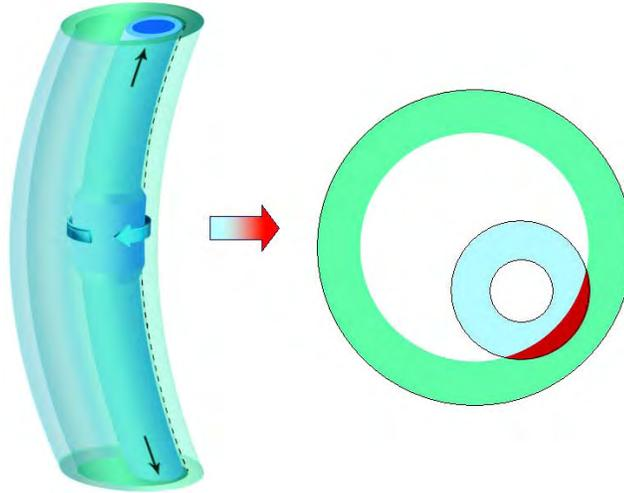
The definition of wear factor is the ratio of friction factor to specific energy, which is the amount of energy required to remove a unit of steel. The unit for wear factor is  $E-10 \text{ psi}^{-1}$ . Therefore, when a wear factor is reported as 8, the actual value used in casing wear calculation is  $8E-10 \text{ psi}^{-1}$ .
