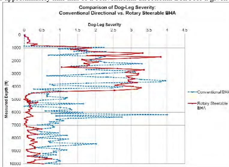
**Figure 4. Graph comparing the dog-leg severity of a conventional directional BHA vs. rotary steerable BHA in similar Gulf of Mexico wells.**
