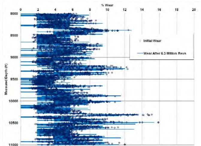
Figure 20. Comparison of casing wear after initial wellbore without NRP use, then after a sidetrack requiring over 6 million revs. With the use of NRP, there is no discernible increase in wear even after 6 million revs.
