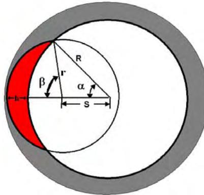
The relationship between wear depth and casing wear volume is:
