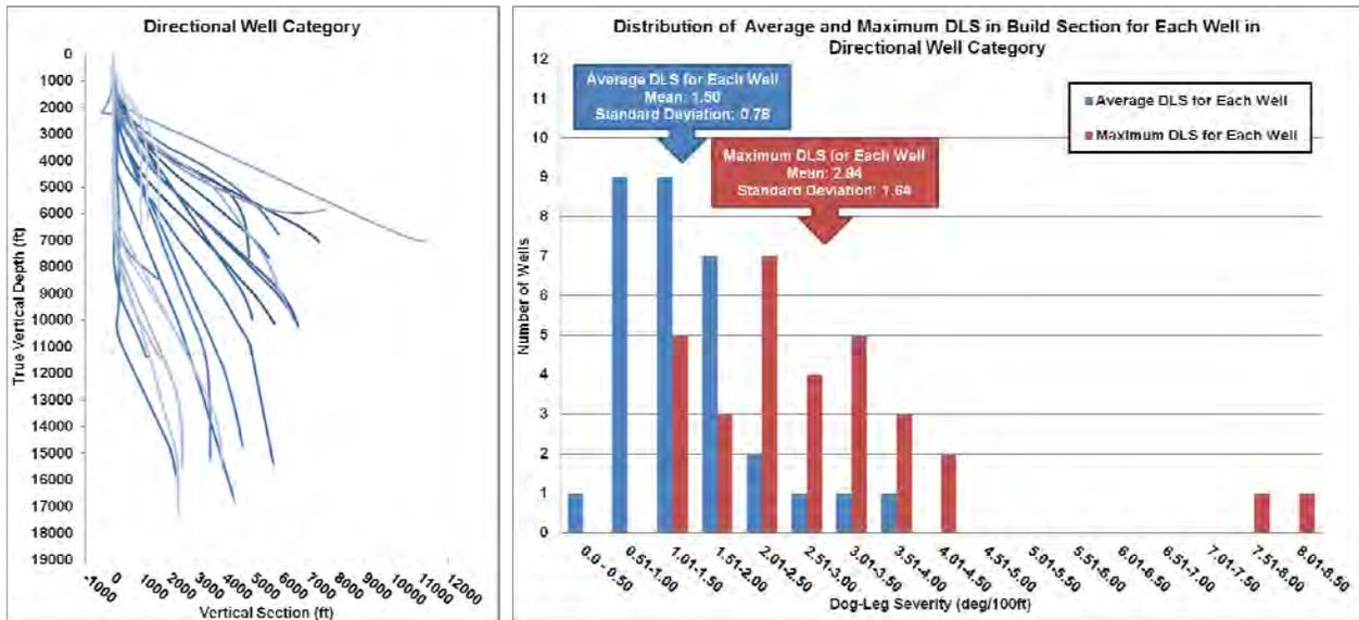
Figures 1 and 2. Chart showing all wells in the directional category, with a histogram of average and maximum dog-leg severity in the build section for each of these wells.
