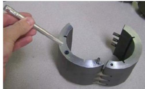
**Figure 3.** Maximum-registering thermometer shown with one half of the encapsulating collar assembly.
