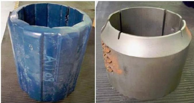
**Figure 1.** The existing design of a high-temperature non-rotating drill pipe protector for cased-hole. Each assembly consists of one rubber sleeve and two aluminum stop collars. The sleeve is “free floating” on the pipe between the two stop collars.
