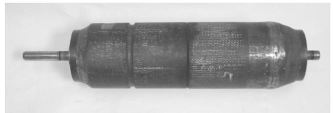
Figure 2. Sample Tool Joint.
