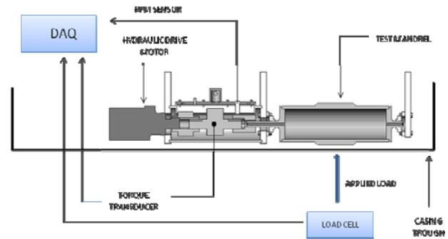
Figure 1. Test Fixture Diagram.
