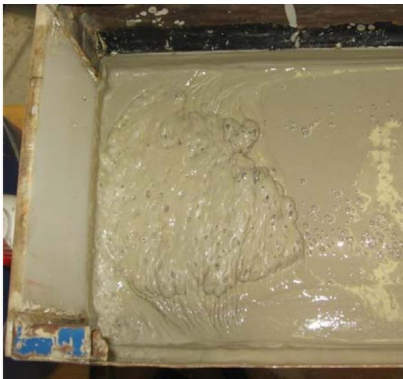
Figure 7. Accumulation of Lubricant Sludge During Lubricant #2 Trial.
