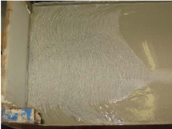
Figure 6. Accumulation of Bead Particulate.
