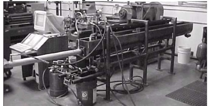
These tests were conducted in an actual segment of 9-5/8” x 47 ppg casing. The casing was new with the I.D. surface left in stock condition/roughness with no polishing or other surface modifications. The data from the series of tests described above was combined providing the average rotational and sliding COFs shown in Table 1:
