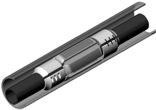
In addition, the Low-Drag NRDPP sleeve utilizes low-friction composite wear pads on the O.D. to significantly reduce the Coefficient Of Friction (COF) between the sleeve and casing wall. The sleeve’s O.D. also incorporates a multi-radius geometry that allows maximum and uniform contact area between the low-friction wear pads and the casing wall, while ensuring adequate passage for drilling fluid flow in order to minimize hydraulic pressure loss across the sleeve. (See Figure 2).
